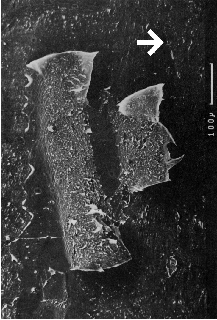
Fig. 11. Combination of macroductile and microductile behavior: failure energy approximately 500 \text{ J m}^{-2} . The arrow indicates the peel direction.
