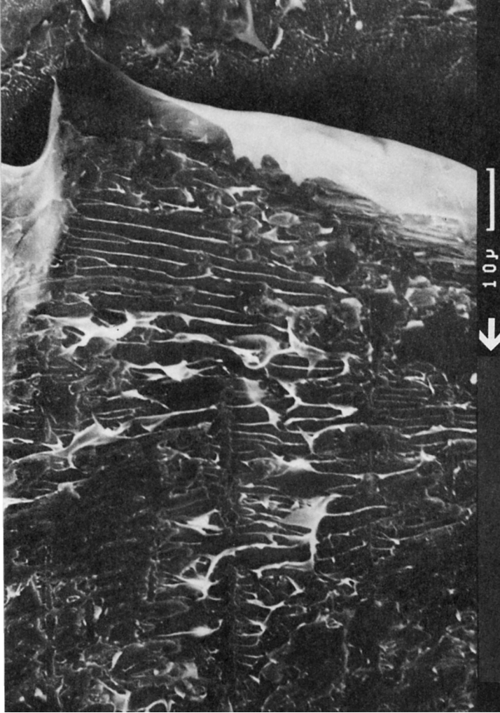
Fig. 12. Macroductile and microductile behavior in an "autohesive" PET laminate. The arrow indicates the peel direction.
